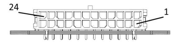
Converter has 12 contact pairs witch are M-BUS interfaces. Converter allows connecting up to 10 M-BUS devices. You can choose any 10 contact pairs. Wherein 1-2 contacts are M-BUS- (bot row), and 13-24 contacts are M-BUS+ (top row).
