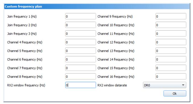
This frequency band allows you to set up to 16 channels, as well as the frequency and speed of the second receiving window.
