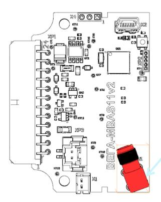
SMA connector for an external LoRaWAN antenna connection
