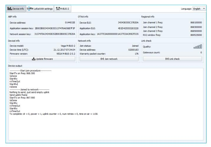
ABP info - displays the data necessary to register the device in the LoRaWAN network with ABP method (Activation By Personalization).
