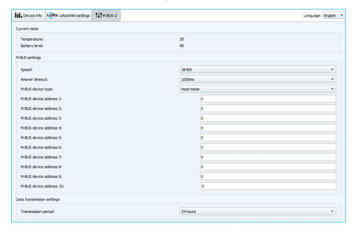
**Current state** – displays the current parameters of the device - the internal temperature of the device and the battery level.
